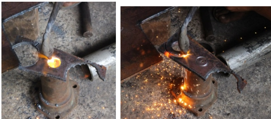
Gambar 4.2 Proses cutting plat besi
