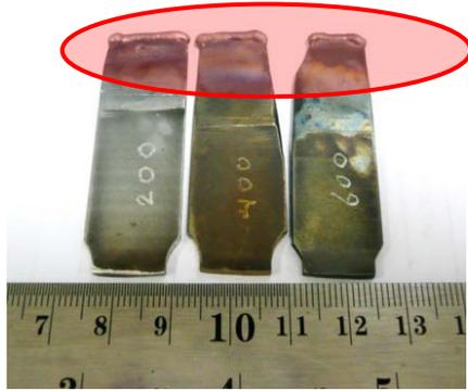
Fig. 6 : Photographs of welded articles, weldments are marked with red circle
