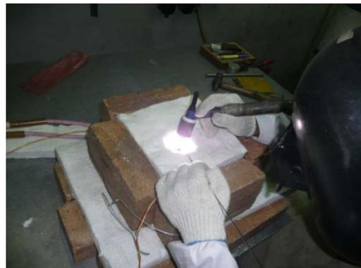
Fig. 5 : GTAW process being performed
