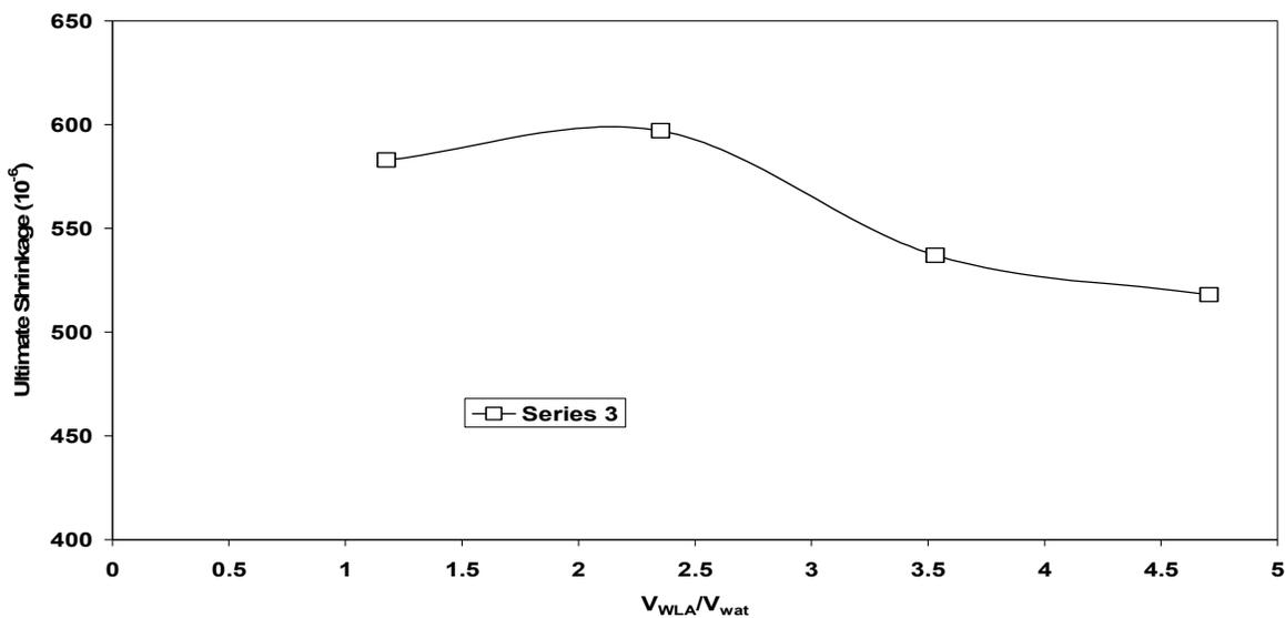
Fig.4. Relationship between ultimate autogenous shrinkage and  $V_{WLA}/V_{wat}$
