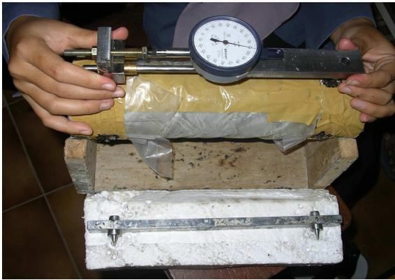
Fig. 1. Measurement of autogenous shrinkage using Demec Gauge
